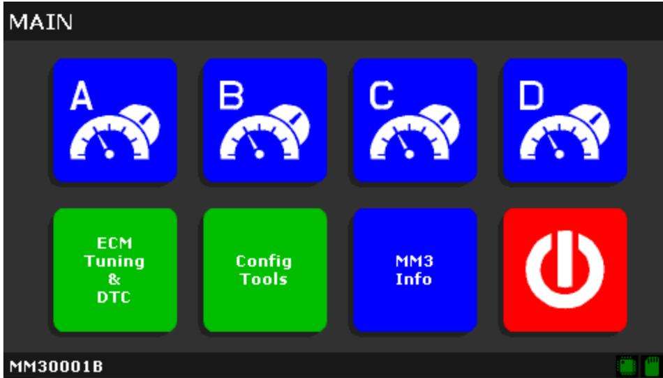
2. Create a stock file for the truck by doing the following: Switch your key to the *ON* position(DO NOT START TRUCK) . Enter the main menu by pressing the (...) button at the top center of the display. Next, select the (ECM Tuning/DTC) select (ECM) then click (Get Stock File For Truck).
